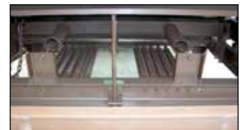
HEAVY-DUTY SPRINGS HELP LIFT THE DECK WHEN A TRUCK COMES INTO CONTACT WITH THE DOCKLEVELER
